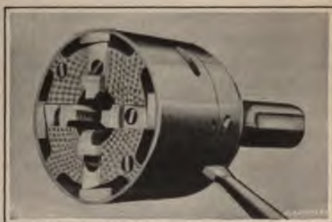
Fig. 8. "Namco" Self-opening Die-head of Non-revolving Type
